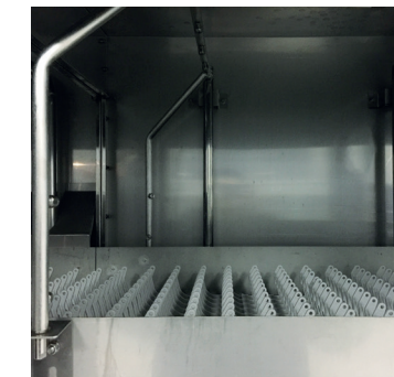
Fully stainless steel rinse circuit
