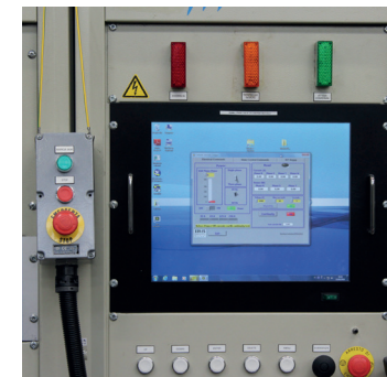
Computer-aided quality testing on all units during production
